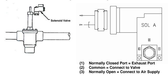
Figure 32: Solenoid Valve Location on Sequence-T Valve & Compressed Air Connections
